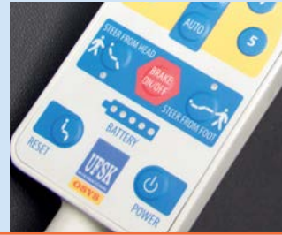
Electronic braking system with "Steering Guide" function acting on all wheels.
