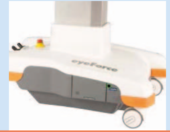
Battery drawer for easy and rapid battery changes.
